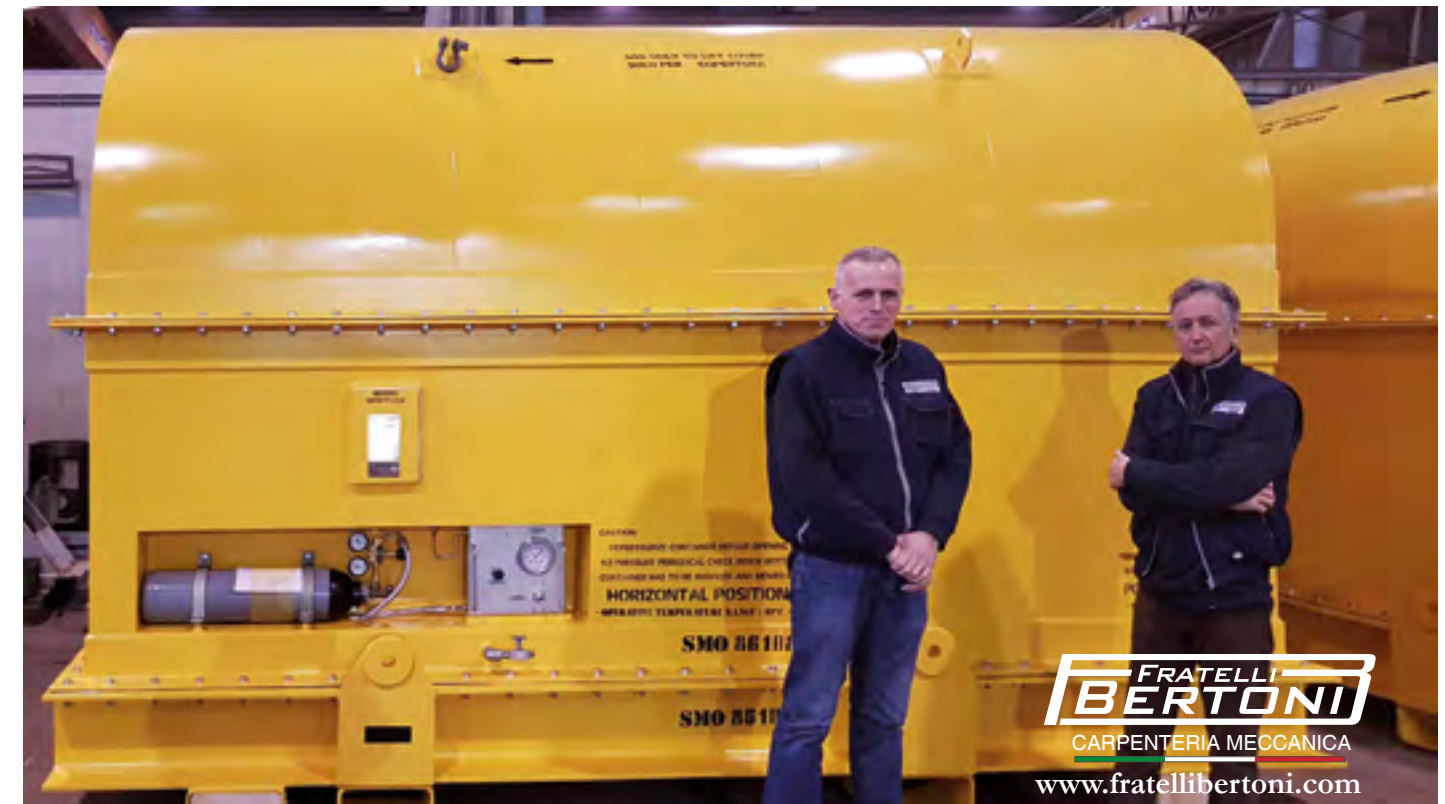
Nitrogen pressurized containers for transport and storage of turbine rotors
